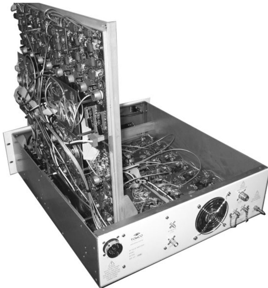
Figure 2 Internal view of Tomco amplifier, showing the two-level foldout shelf arrangement.
